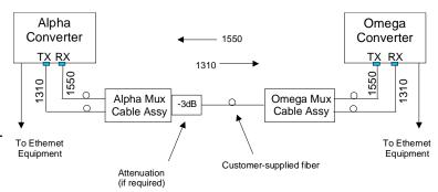
The kit combines the transmit and receive signals onto a single fiber. Two special, media converters are connected to the single fiber via two, different, Mux Cable Assemblies. The kit sends 1310 signals in one direction, while 1550 signals travel in the opposite direction. The signals are multiplexed by WDMs, which are built into the Mux Cable Assembly. Eventually, each end's components will be built into an enclosure. This enclosure will have only one fiber connection.
