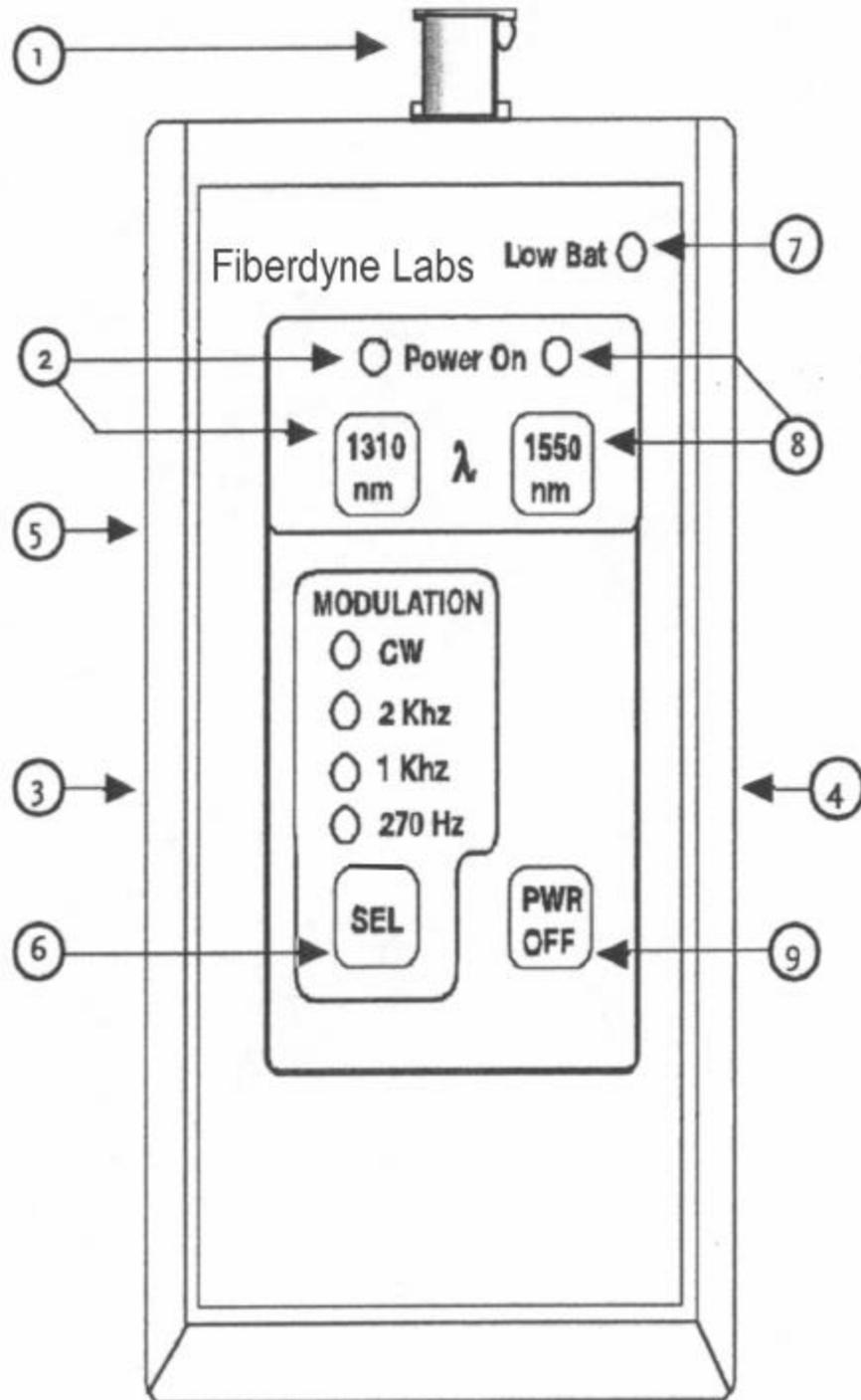
Figure1- FD-FS1316Fiber Source Front Panel
