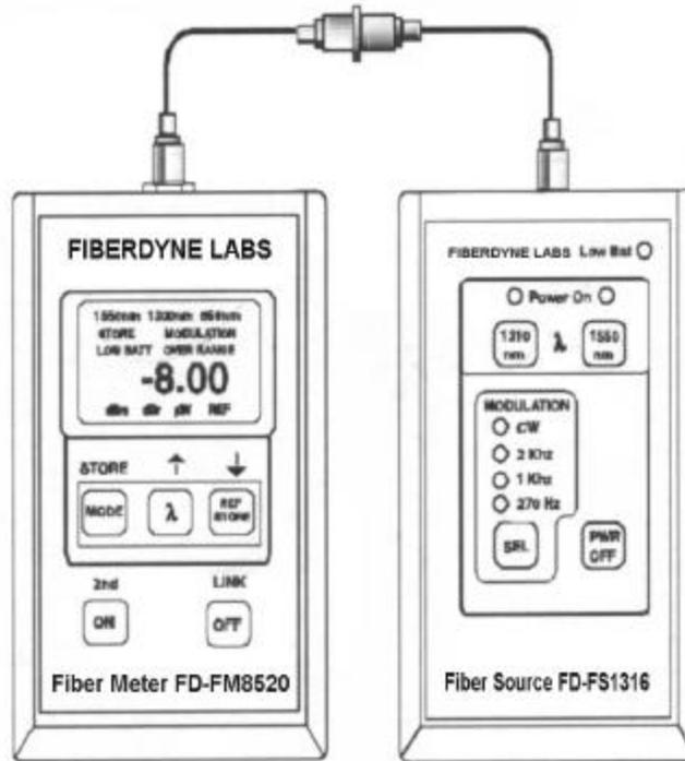
Figure 2 – **Optical Power Verification Diagram**
