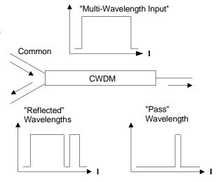
wavelengths will include eight wavelengths, from 1470 to 1610. The center of each pass band is spaced at 20 nm intervals (e.g. 1530, 1550, 1570, etc.).
