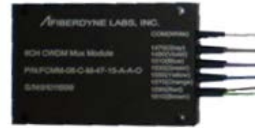
Field module with 900um pigtailed
